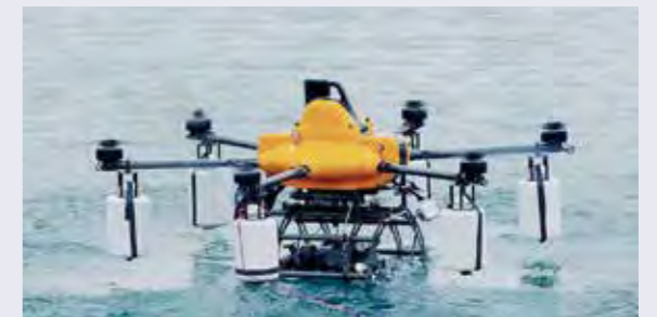
"Amphibious drone" to be used for underwater inspection work, etc.
