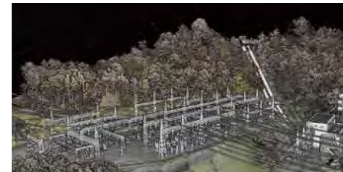
Example of 3D modeling from drone-captured data: Nukabira Power Plant
