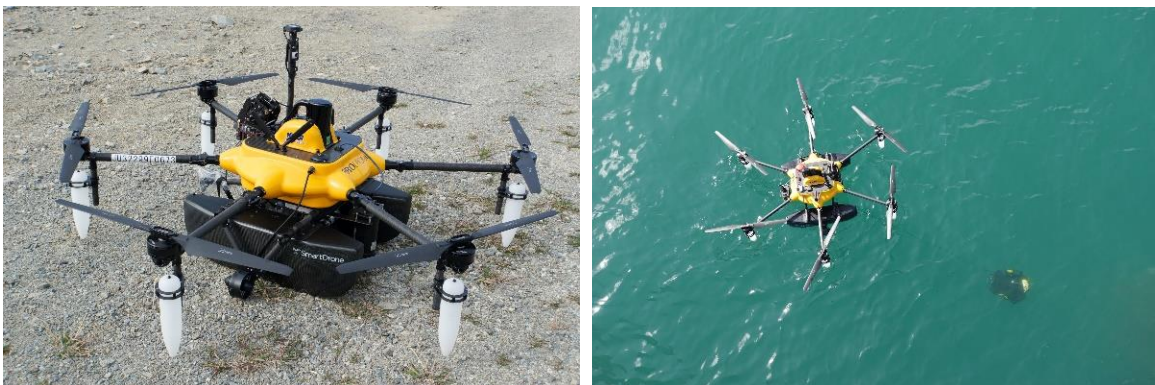
Fig. 18 Base unit (left) The sub-unit separates from the base unit and dives underwater (right)
